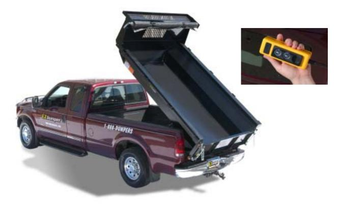
EZ Dumper dump trailers and dump inserts for pickup trucks are hydraulically powered. Just push the button on the remote control and the bed raises to an angle of 47° in under 30 seconds for quick and clean unloading.
